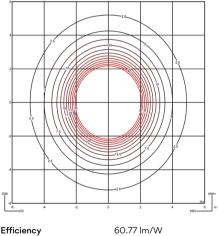
Efficiency Coordination System CG 1607.97 lm **Total Flux** Maximum Value 686.66 cd
